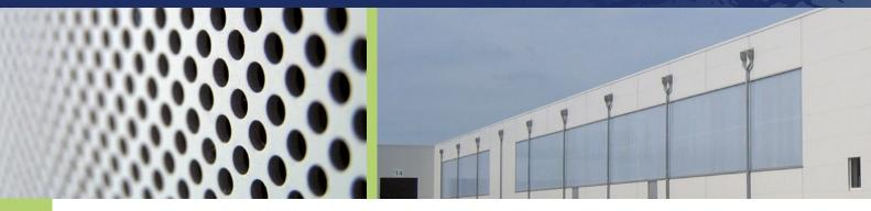
Hipertec® Wall Sound is a sandwich panel with an insulation core of mineral wool and steel cover sheets, the internal sheet being perforated. This panel is perfectly apt for buildings with high requirements for noise insulation and sound absorption. The design of the internal sheet improves room acoustics substantially. This system patented by Metecno applies a special fleece as trickle pro-
